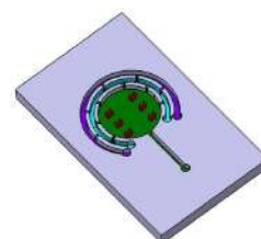
(A) Molecular model of nanoparticle transport in cell membranes, (B) Biomimicking tumour-on-chip microfluidic platform for validation of molecular model
