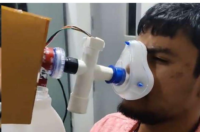
Inexpensive Portable CO 2 -oximetry device for in-home/Remote Cardio-pulmonary status assessment
